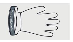
Replace silicone band with o-ring in groove on suit ring. Put suit on before attaching dry gloves. Squeeze the glove ring and suit ring together to seal.
